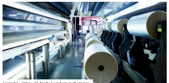
Secondary slitter with finished products in the factory
